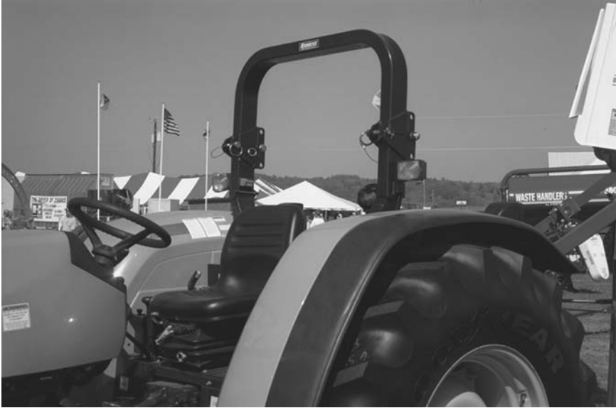
FIGURE 6.2. Two-post folding rollover protective structure (ROPS) in upright position.
